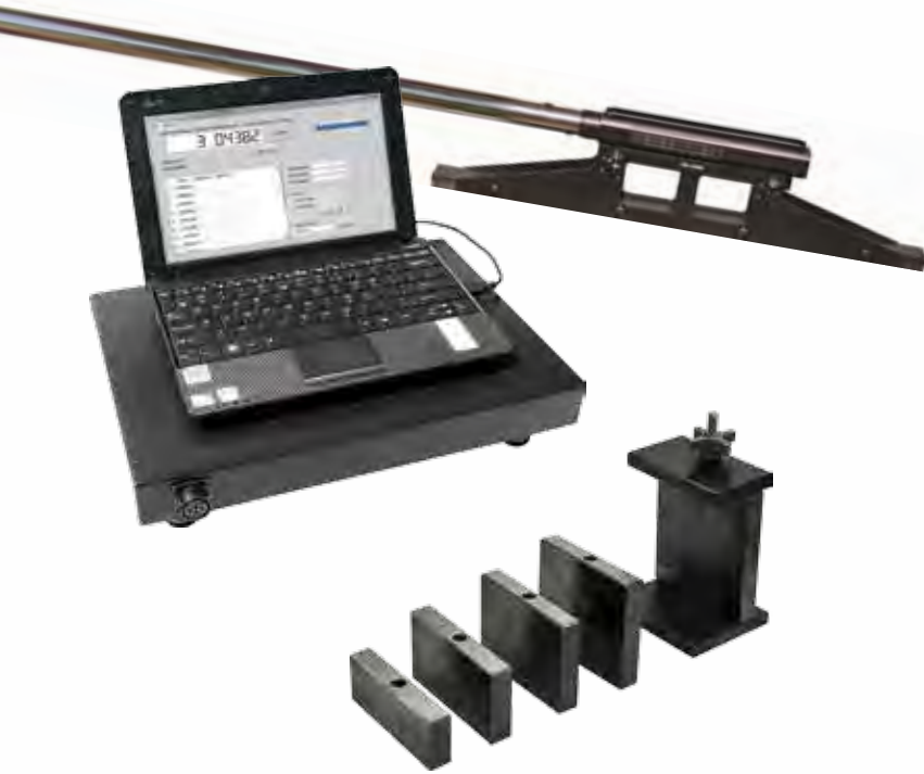
Stator Bore Diameter Measurement
